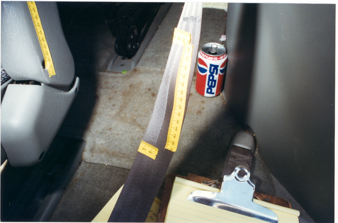
102. Close-up of an abrasion on the restraint webbing caused by the plastic cover.
